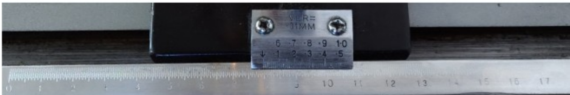
Figure 4: Vernier Scale of the Microscope
